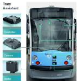
2016: Product: Siemens Tram Assistant (based on BOSCH TFCW); Den Haag, Ulm, Bremen, ...
